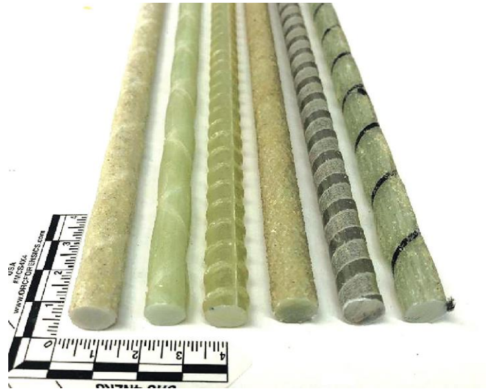
Figure 1. Types of FRP bars predominantly used in building and construction.
